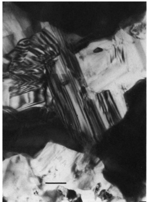
Fig. 6. TEM micrograph of a \text{Si}_3\text{N}_4 /TiC composite showing the reaction zone. Scale bar = 0.2 \mu\text{m} .
