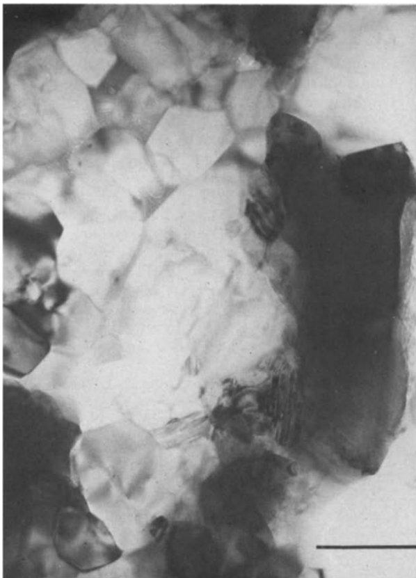
Fig. 10. TEM micrograph of a \text{Si}_3\text{N}_4/\text{TiC} composite crept at 1340^\circ\text{C} for a stress of 200 MPa up to 15% deformation showing the absence of microcracks and cavities. Scale bar = 0.5 \mu\text{m} .
