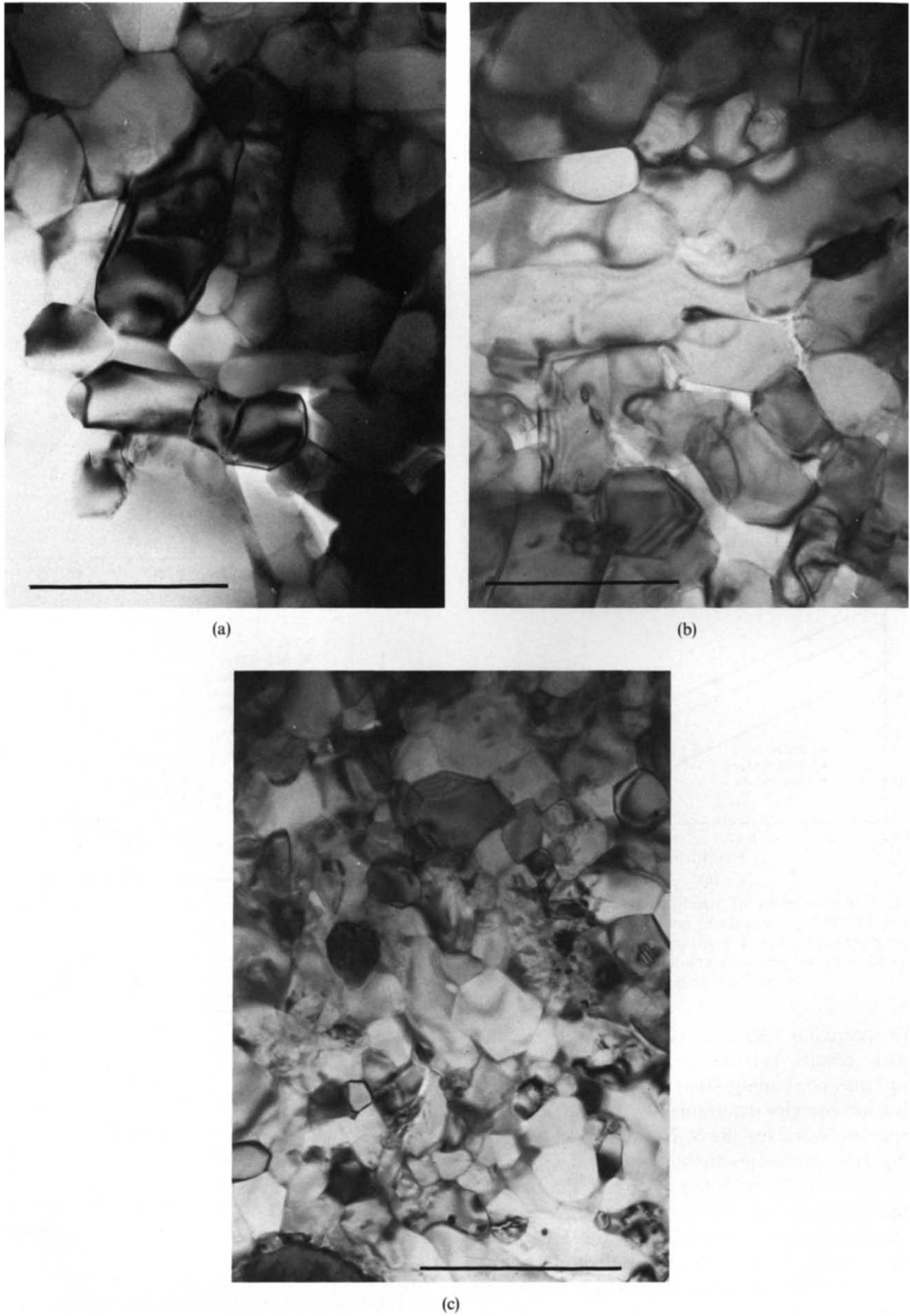
Fig. 3. TEM images of (a) the dispersoid-free, (b) 40 wt% TiN-Si 3 N 4 and (c) 40 wt% TiC-Si 3 N 4 matrices. Scale bar = 1 \mu m.
