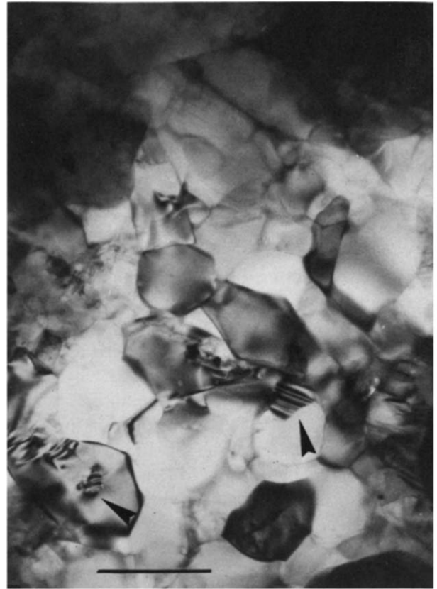
Fig. 5. TEM micrograph of the \text{Si}_3\text{N}_4 /TiC composite showing the matrix polluted by SiC precipitates. Scale bar = 0.5 \mu\text{m} .
